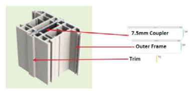
As you can see in this diagram, the coupler is inserted between two pieces of outer frame profile and acts as a joiner. The gap which is caused by the coupler is concealed by a piece of trim.
