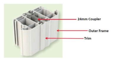
As you can see in this diagram, the coupler is inserted between two pieces of outer frame profile and acts as a joiner. The gap which is caused by the coupler is concealed by a piece of trim.
