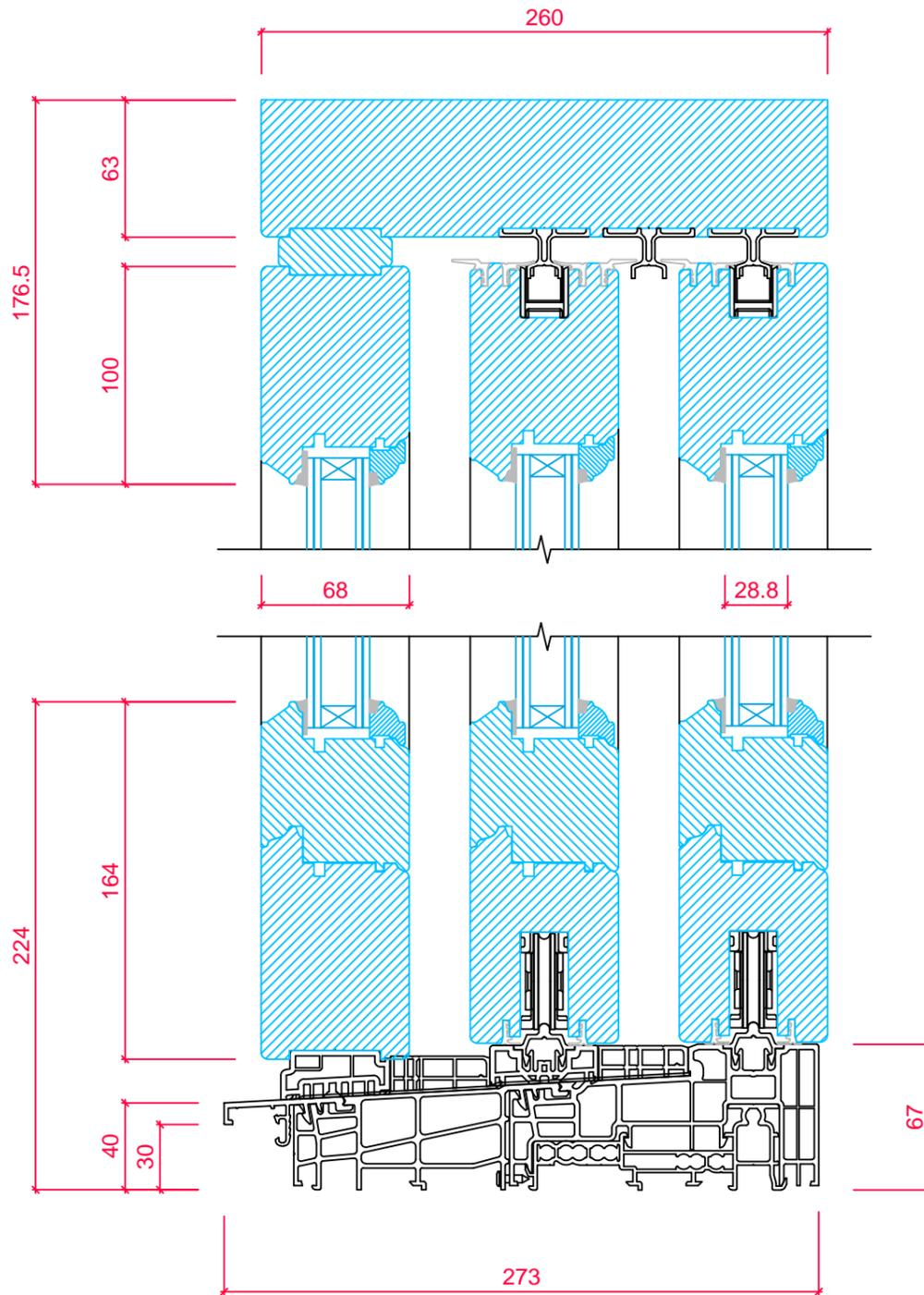
**FRAME CROSS SECTION 'A-A'**
